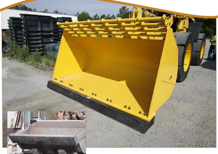
SETCO's rubber cutting edges are made from durable natural rubber that unlike steel, will not wear out your concrete and will not spark. The rubber also acts as a sponge that keeps the floor drier, thereby increasing the traction of solid tyres. Tapered on both sides, the rubber cutting edges are even reversible!
