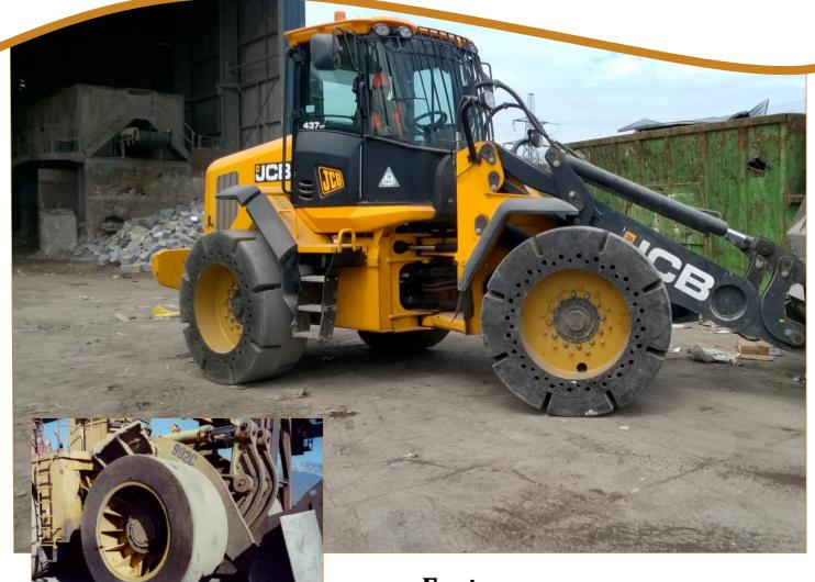
SETCO's expanded rim solid tyres are designed for the toughest environments were traditional press-on tyres would fail. Using 100% natural rubber for its superior wear and cut resistance, SETCO's expanded-rim solid tyres will withstand even the toughest load and carry scrap and waste operations.
